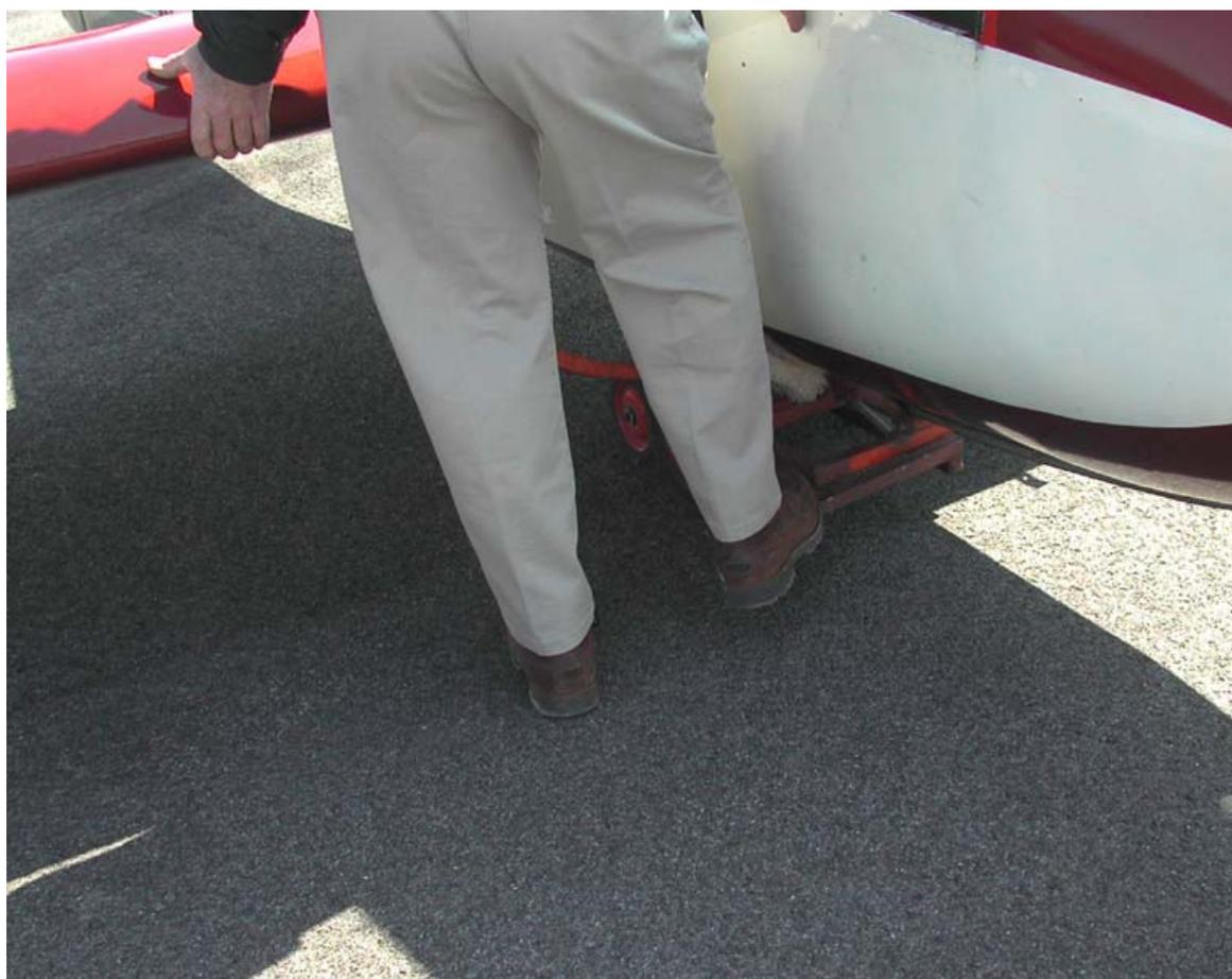
After the fuselage is lifted from the dolly, leave your foot on the lever and push back on the wing until the fuselage is separated from the dolly.
