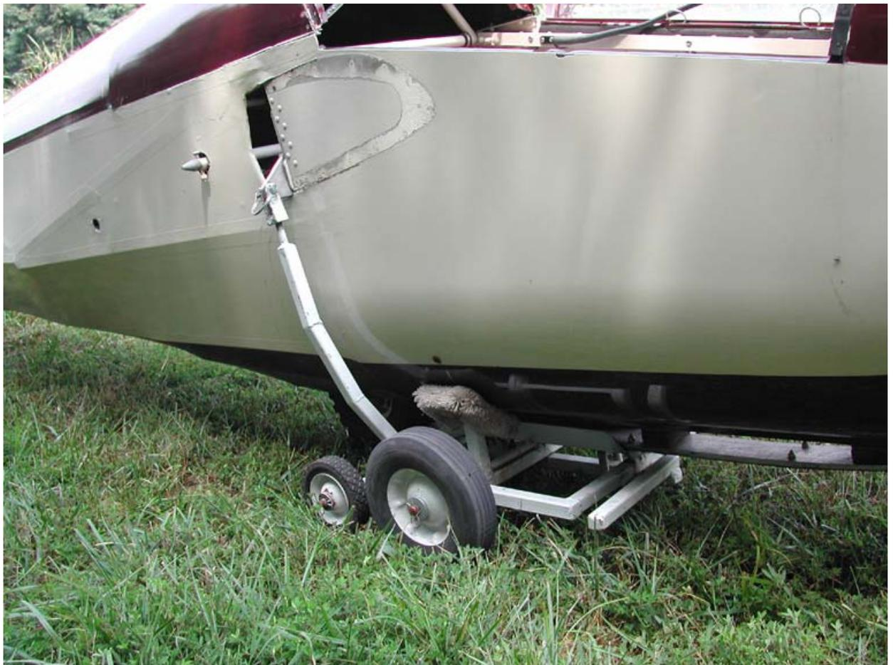
6. A foot operated lever with a roller wheel in contact with the skid lifts the skid up from the dolly channel and permits the fuselage to be up from the dolly. The roller wheel lever applies about a 10 to 1 mechanical advantage, so you will be exerting about 40 pounds of force to lift the fuselage from the dolly. This allows the fuselage to clear the two saddle pads and the channel that supports the skid. The picture shows the lever lifting the fuselage.
